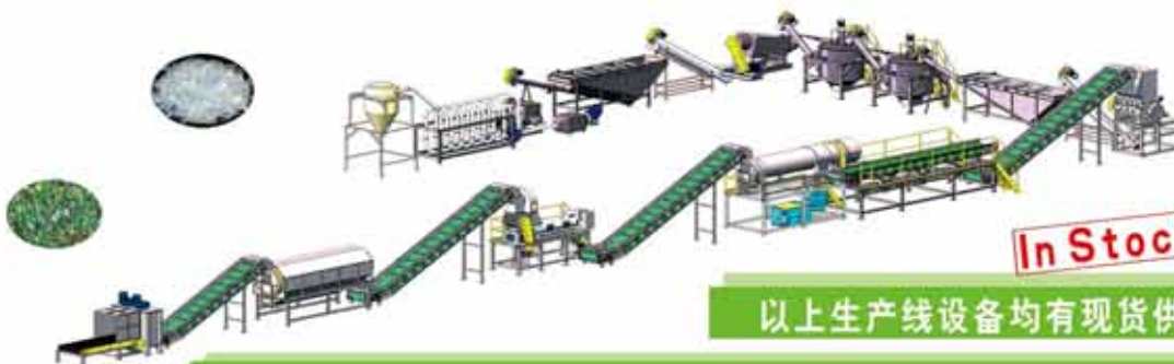
PET瓶破碎清洗脱水及干燥生产线 PET Bottles Crushing, Washing, Dewatering and Drying Line
