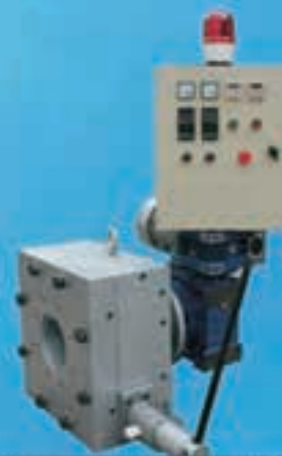
Melt Filter without Wire Mesh
