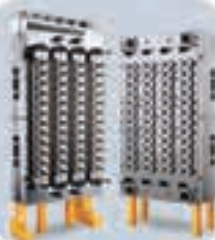
48 CAVITY HOT RUNNER PREFORM MOULD
