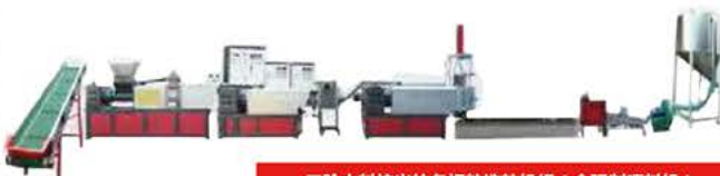
三阶段水料挤出拉条切粒造粒机组 (含强制喂料机) Third-order water extrusion stripping pelletizing granulation unit (including forced feeder)
